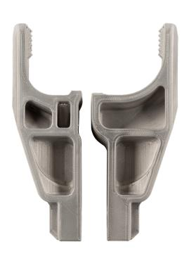
By printing the mounts from high-temperature PEEK filament, they will be able to withstand the environment inside the system - which includes hot welding slag, sparks and parts being dropped, helping to reduce downtime the results from damage to sensors.
