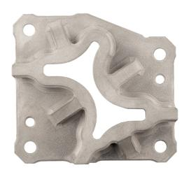
Today, the vast majority - as much as 80 percent - of Egar's 3D printing capacity is dedicated to producing end of arm tooling for their high-volume production stamping presses. Using just one Studio System, staff can design, iterate, and integrate components into their production line in less than a week - keeping manufacturing downtime to a minimum.
