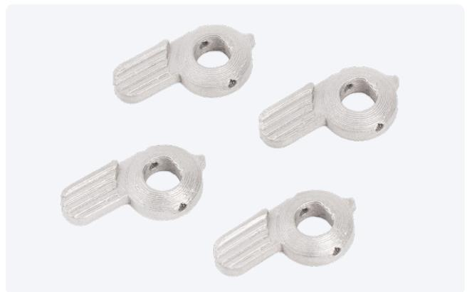
Created to allow customers to validate part designs before investing in tooling, these parts also helped Ecrimesa validate the capabilities of the Studio System.
