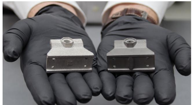
— A custom mounting bracket 3D printed on the Desktop Metal Production System P-1 in under two hours. The as-printed part, above left, was then blasted with alumina grit for the final surface finish, above right.
