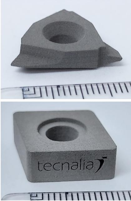
M2 tool steel cutting tool inserts produced with binder jet 3D printing by TECNALIA
