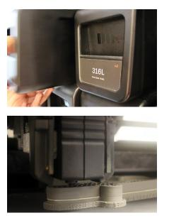
Bound Metal Deposition technology extrudes pre-bound metal rods from easy-swap cartridges, top, into complex shapes to build parts layer-by-layer. The white ceramic interface, seen above, allows the final part to easily break away from any support structures after sintering.
