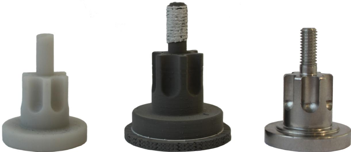
“Zero-type” parts, left, are 3D printed in plastic on ETEC digital light processing machines to test for fit and function. Designs are quickly advanced to functional prototypes. The green part, center, is 3D printed in metal on the Desktop Metal Studio System with ceramic interface for sintering to support the printed threads. The 316L stainless steel end-use part, right, in finalized within weeks, compared to 54-58 weeks for traditional production.
