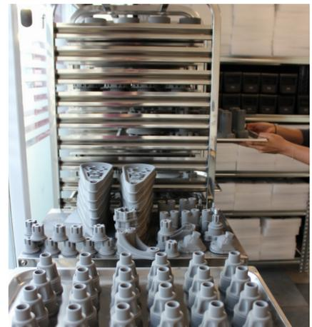
“We’ve measured one degree of heat exchange as fish are processed through the filleter,” he explained. “Heat increase means degradation and a shorter shelf life. By incorporating internal cooling channels within the components, we’re able to negate that and help keep the fish fresh. We have been increasing the yield and increasing the freshness,” Hreinsson said.
