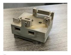
The flexibility of Desktop Metal BMD technology allows Burke Aerospace to produce a variety of complex fixturing designs with ease.
