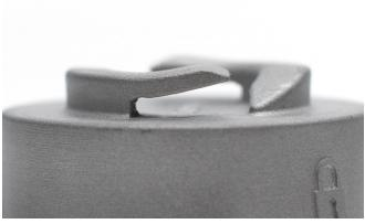
The overhang of the connector on the left sags in the furnace without sintering supports. The overhang on the right, run through Live Sinter to simulate the warpage and distortion during sintering, was 3D printed with a negative offset geometry that sinters to the final specification.
