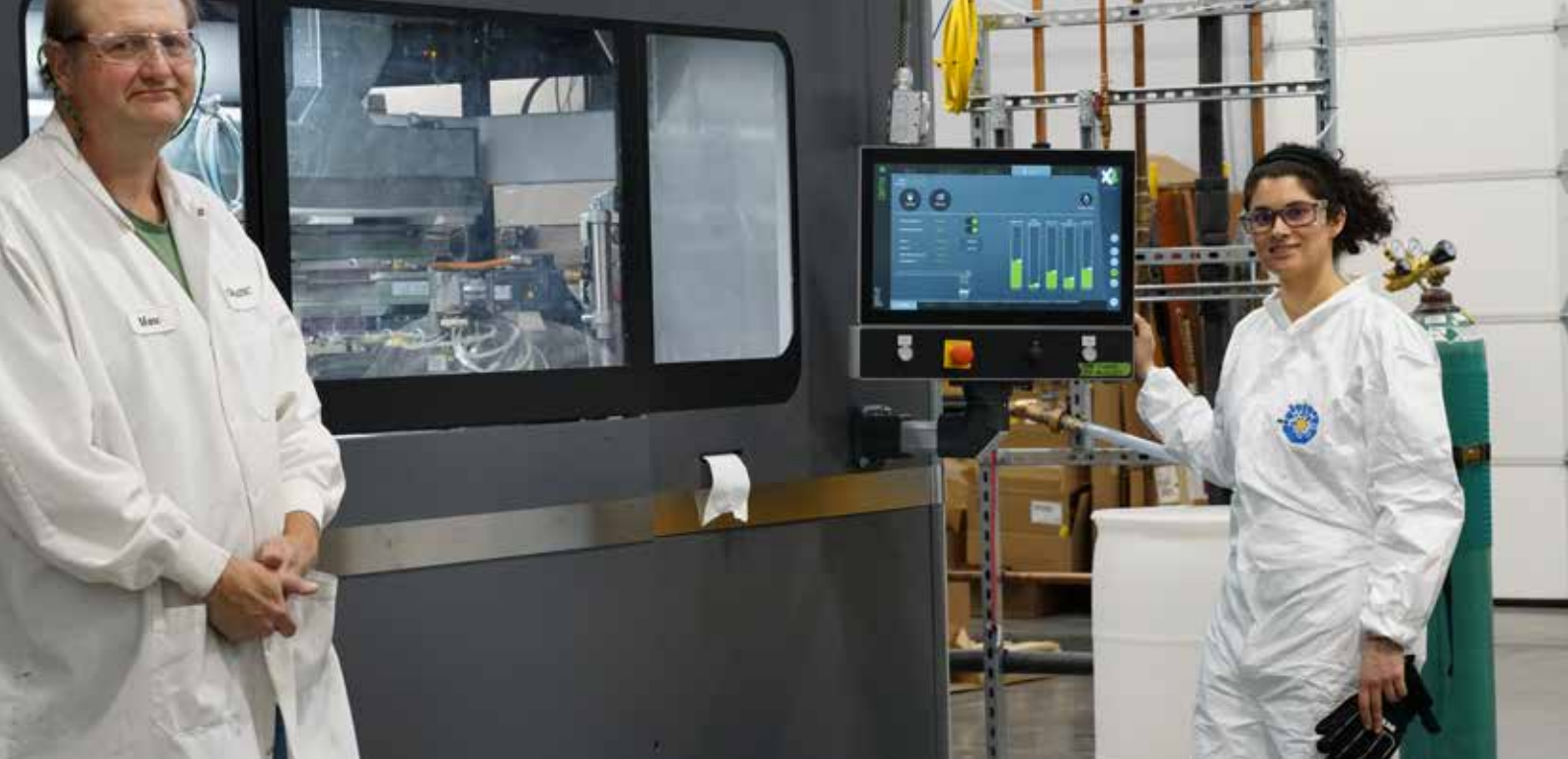
Pictured above, employees of Ultra Safe Nuclear Corporation with a Desktop Metal X160Pro being used for Silicon Carbide production used in USNC's Fully Ceramic Micro-encapsulated (FCM) fuel. The manufacturing of FCM is enabled by Desktop Metal binder jet 3D printers and their ability to 3D print silicon carbide heat-resistant ceramic particles in unique geometries that can safely surround a standard type of nuclear fuel particle known for its safety.
