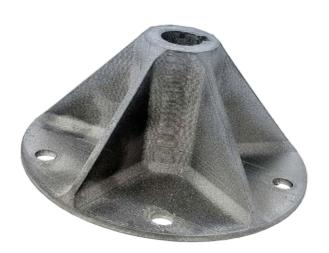
This wheel hub was 3D printed in stainless steel on the Desktop Metal Studio System. The motor-to-wheel hub interface required the ability to endure high torque loads and harsh environmental exposure. The inhouse 3D printed components met the structural requirements and significantly reduced secondary machining operations and turnaround time. stack-ups.
