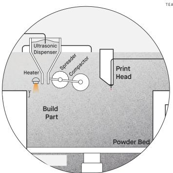
Triple ACT features an ultrasonic dispensing system for consistent flow of fine powders with a spreading roller system and counter-rolling compactor for high green strength
