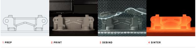
Secure, web-based software constructs build plans from STL or CAD files, automatically generating supports and control parameters based on part geometry and material.
