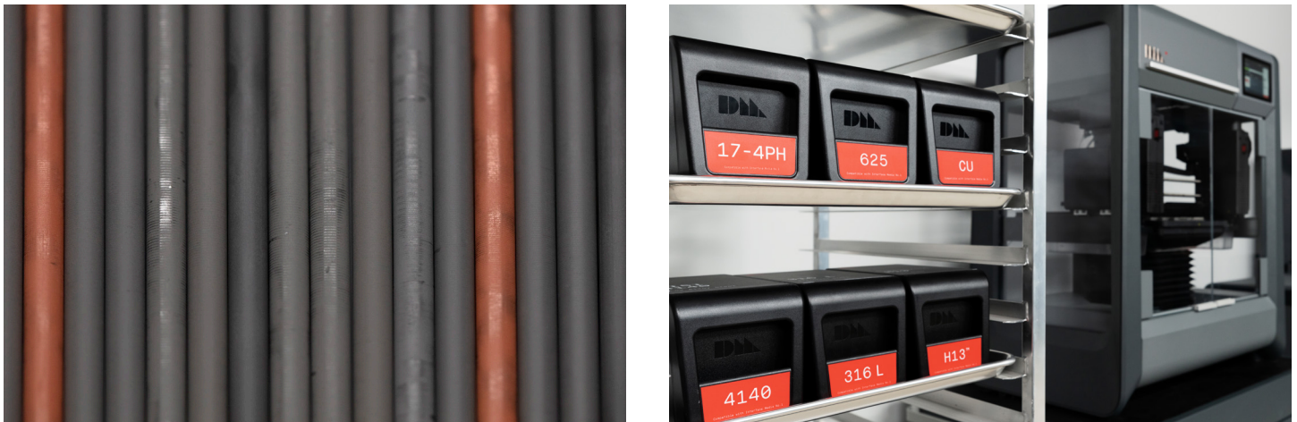
Left, pre-bound rods of metal and binder for the Desktop Metal Studio System, seen at right with a variety of material cartridges that make for easy machine operation and material changeover.
