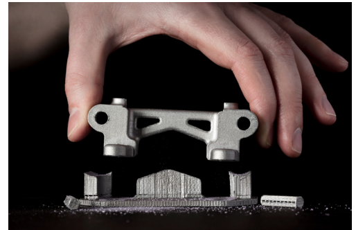
Supports printed on the Studio System break away by hand after sintering, allowing for easy post-processing of Bound Metal Deposition prints.
