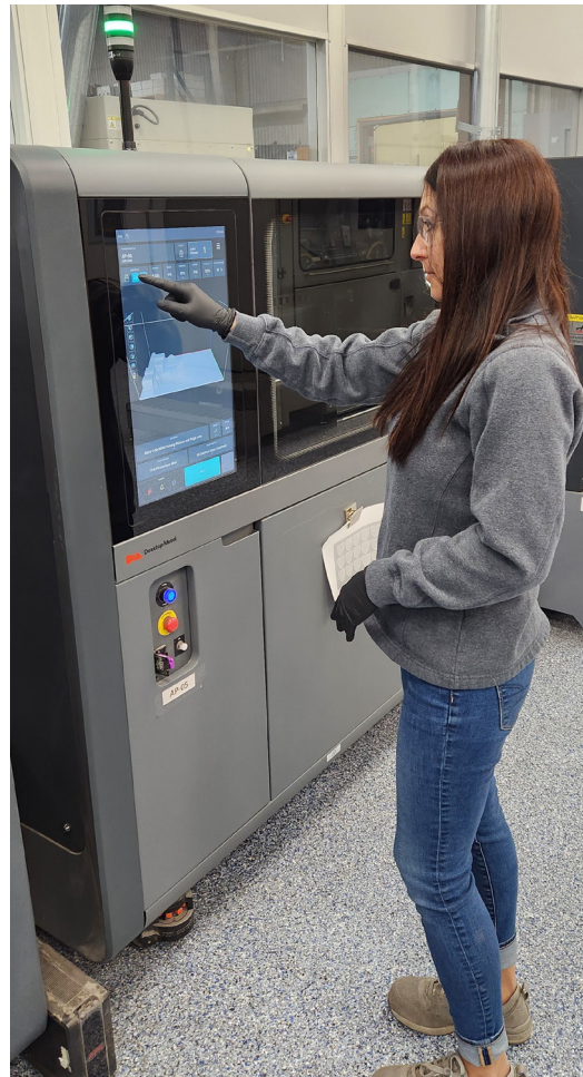
The APG team operates powder-less metal 3D printing on the Studio System, far left, and increases throughput with binder jetting technology on the Shop System, left.
